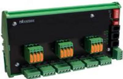
The TELEM family RTU module TELEM-AI12-T with 12 analog differential analog inputs is used for measure 12 analogue values. Module bases on 32-bit ARM CPU. Interfaces to other equipment are RS-232 and RS-422/485. Data exchange protocol is IEC 60870-5-1-101.
