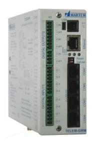
Telem-GWM-C1-B is a modification of Telem-GWM to be used in places with no low voltage electricity. It is powered from accumulator which is charged by high voltage measurement transformers.
