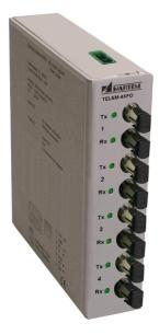
Telem-4xFO is used for building up point-tomultipoint optical communication line. Master device is connected via RS-232 or optical interface. Remaining optical interfaces are connected to slave devices. For increasing the number of slave channels the Telem-4xFO modules can be stacked together via RS-232 interface.
