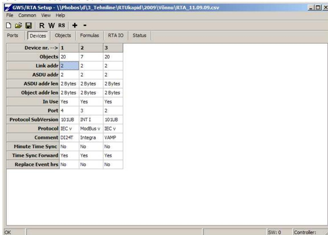
Up to 20 downlink devices can be connected to GW5 and configured on this tab card.
