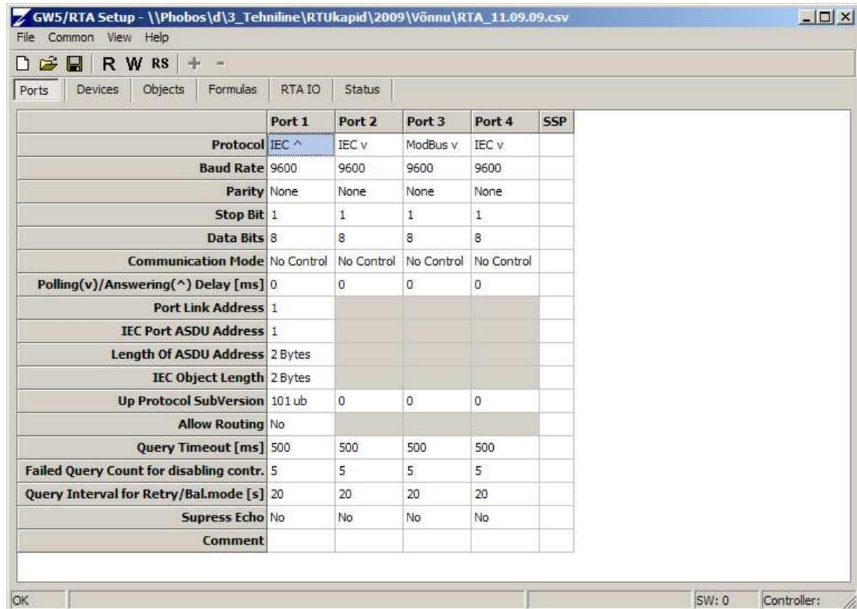
From the **View** menu a **Basic** or an **Advanced** view of the **Port configuration tab card** can be selected. The advanced view shows the additional query and echo suppression parameters.
