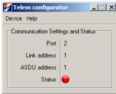
Warning **Check communication** – If there is no connection with the RTA device then the warning message is displayed together with an alarm beep.
