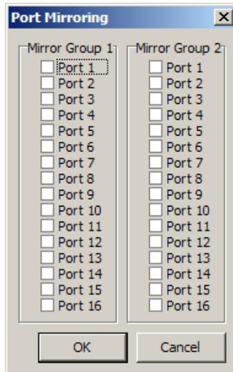
Two redundant (mirror) groups can be configured. The marked ports of one mirror group share the same event buffer. So if the upper level channel is switched over to another redundant channel then there will be no double events.
