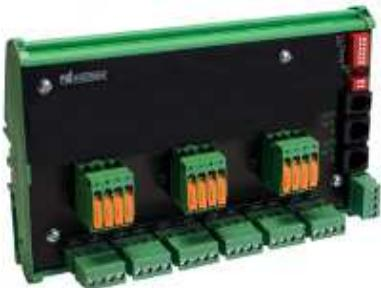
The TELEM family RTU module TELEM-AI12-T with 12 analog differential analog inputs is used for measure 12 analogue values. Module bases on 32-bit ARM CPU. Interfaces to other equipment are RS-232 and RS-422. Data exchange protocol is IEC 60870-5-1-101. Time synchronization is possible with 1 second synchronization pulse and over protocol.
