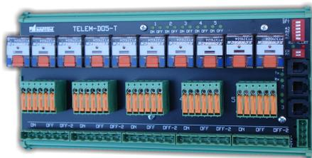
The TELEM family RTU module TELEM-DO5-T with fixed or changeable relay outputs for control operation of 5 objects (+ 3 objects with external relays). The module is based on 32-bit ARM CPU. Interfaces to other equipment are RS-232 or RS-422. Data exchange protocol IEC 60870-5-1-101.
