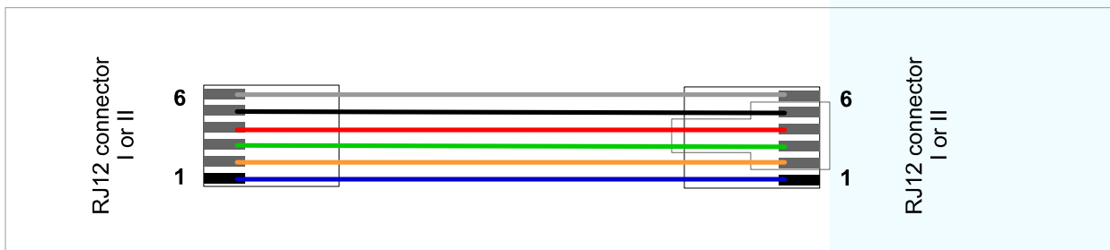
Fig. 6 Cable between Telem4xFO-3 modules
